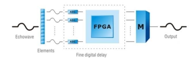
Accurate beam forming and signal processing, digital image acquisition and processing ensure images with clear-cut edge and no distortion.
